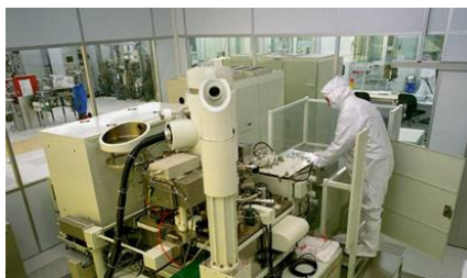
Electron beam lithography system for patterning of nanostructures at Chalmers University of Technology
