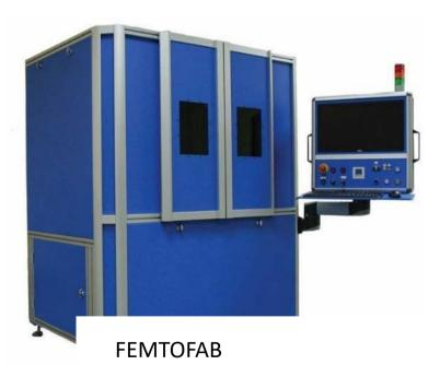
Laser micromachining system, designed for a specific industrial process
