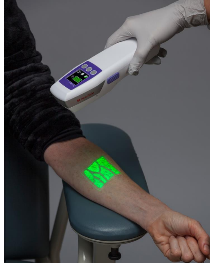
AccuVein AV500 projecting an image on veins AccuVein AV500 projecting an image on veins
