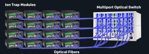
This modular approach allows for indefinite scaling of individual QPUs to form a more powerful quantum system. Reconfigurable multiport optical switch allows for full modular connectivity between all qubits.
