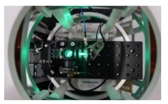
Sensor for measuring finest signals in magnetic fields.
