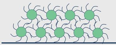
**Colloidal QDs dispersed in solution** are dispensed on wafer by spin-coating
