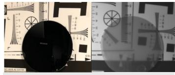
Silicon is transparent to SWIR light enabling SWIR imaging through Si based devices
