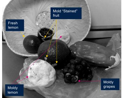
Mold and mold "dust" turns white while the fresh fruits turn dark @1400 nm
