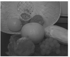
At 940 nm NIR image sensor shows no major contrast. Mold in grapes not visible at all
